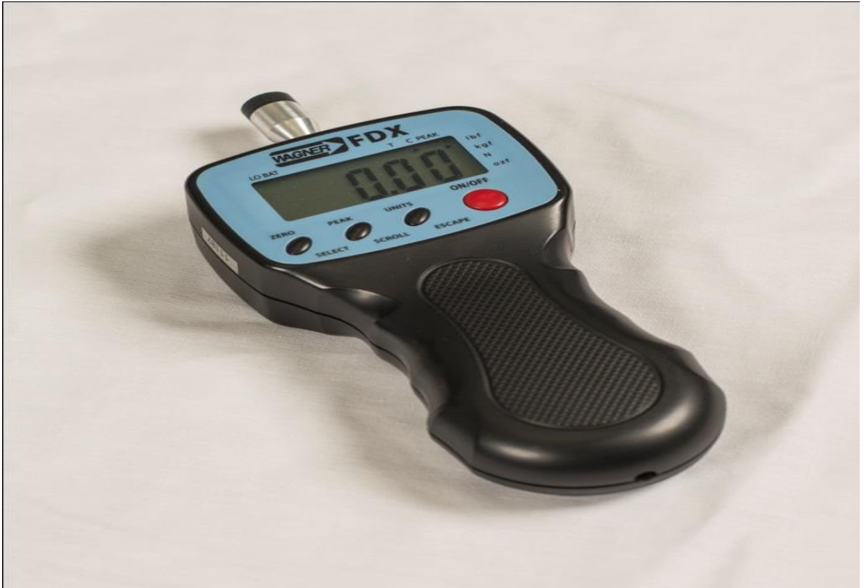
Figure 2. Handheld Pressure Algometer (PA)
